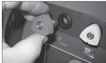
Figure 6 - Insert spray nozzles into the holder
