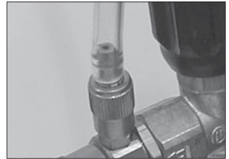
Figure 5 - Attach suction tube to barb fitting
