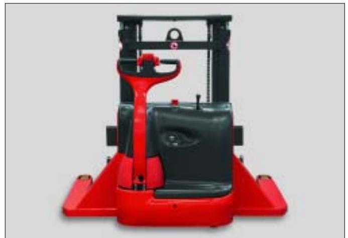
The **L10AS/L12AS** stackers are equipped with straddle legs which allow to pick up and stack all types of loads such as box pallets, gitter boxes or closed pallets. The width within the forks can be adjusted thanks to an ISO fork carriage. The ISO fork carriage can also fit specific applications by adding optional accessories such as grippers or side-shifters.
