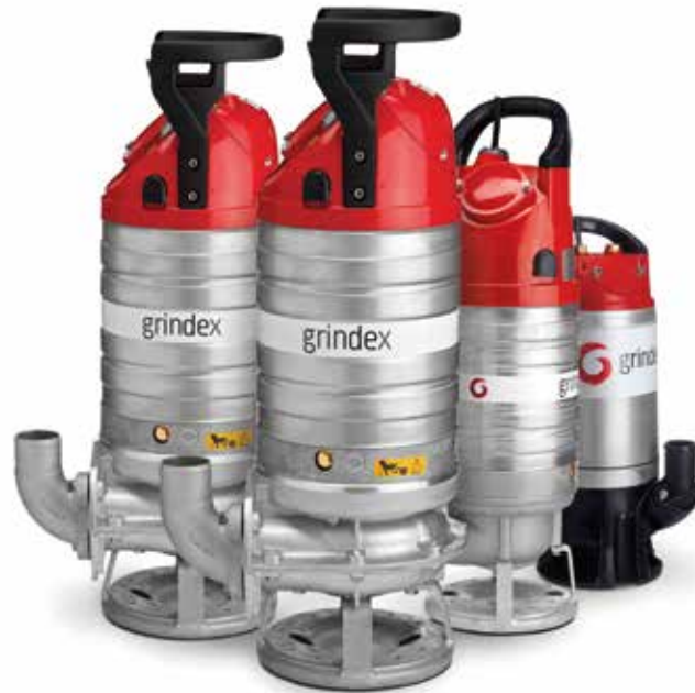
The sludge pumps are built to handle contaminated water, pH 5-8, and water containing relatively abrasive solids up to the size of 3.2 inches.
