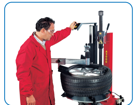
➤ Mounting the wheel with the aid of the bead presser arm
