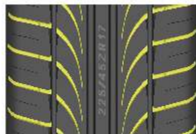
Continuous, solid central rib transfers lateral forces to help provide excellent stability at highway speed.
