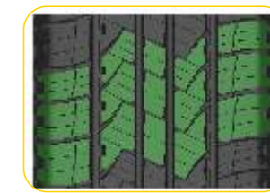
High Density Zig-Zag Siping
