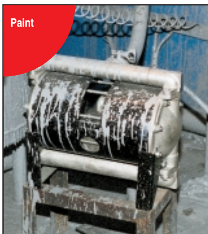
An ARO 3:1 Power Pump circulates injection molding colorant.
